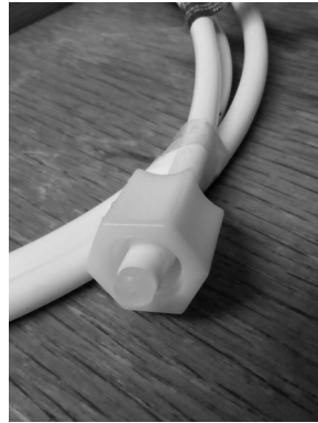
Flow restrictor in situ (drain outlet on membrane)
