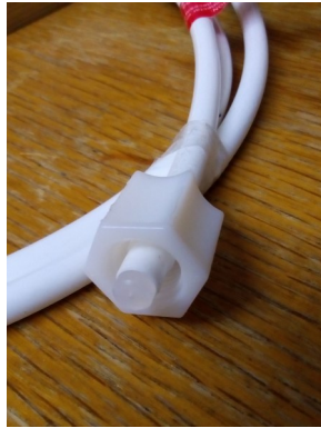
Flow restrictor in situ
